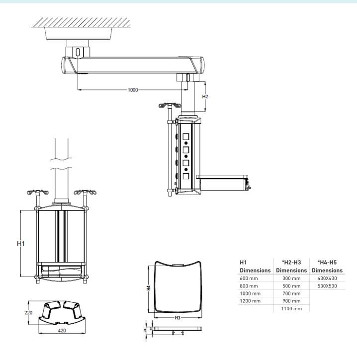
+ Note:  $\pm$  25 mm tolerance is given for metric measurements and  $\pm$  5° tolerance is given for angle measurements.
