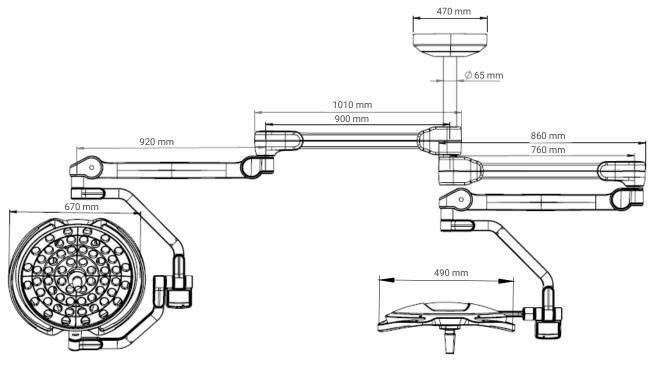
Note:  $\pm$  25 mm tolerance is given for metric measurements and  $\pm$  5°tolerance is given for angle measurements.
